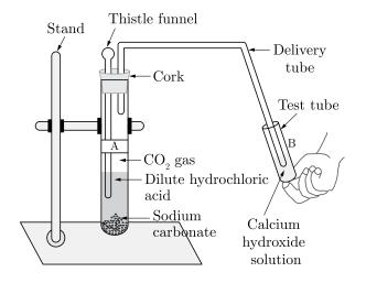
Student takes about 0.5 g of sodium carbonate ( $Na_2CO_3$ ) in test tube A and about 0.5 g of sodium hydrogen carbonate ( $NaHCO_3$ ) in test tube B. After this student add about 2 ml of dilute HCl to both the test tubes.
