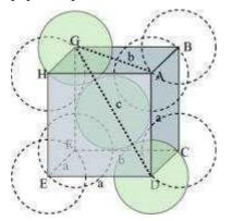
It can be observed from the above figure that the atom at the centre is in contact with the other two atoms diagonally arranged.
