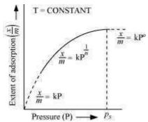
The plot between the extent of adsorption m against the pressure of gas (P) at constant temperature (T) is called the adsorption isotherm.
